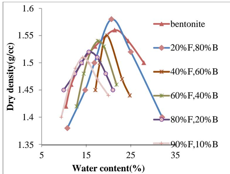
Figure 11: Modified proctor compaction test of expansive soil stabilized with fly ash
