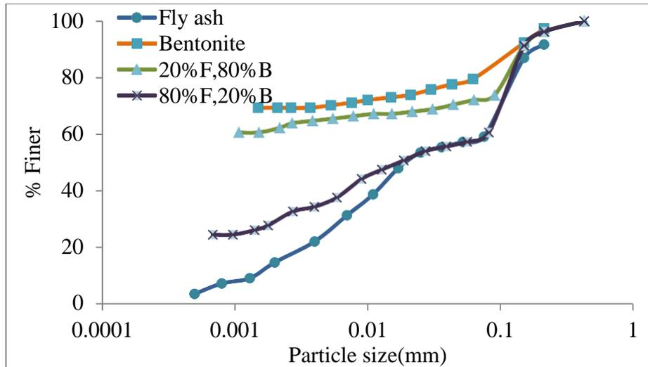
**Figure 9:** Grain size distribution of fly ash and clay
