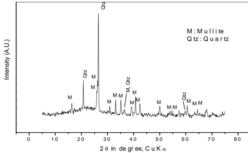
**Figure 3:** X-Ray diffractogram of fly ash
