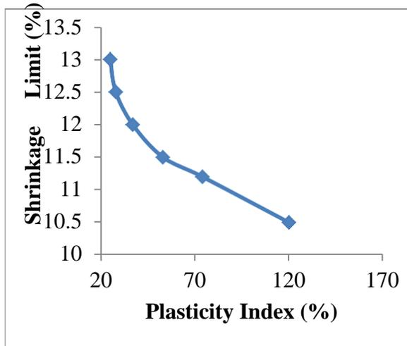
**Figure 6:** Variation of shrinkage limit with PI (%)
