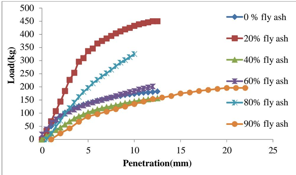
**Figure 18:** Unsoaked CBR test result expansive soil mixed with various proportion of fly ash
