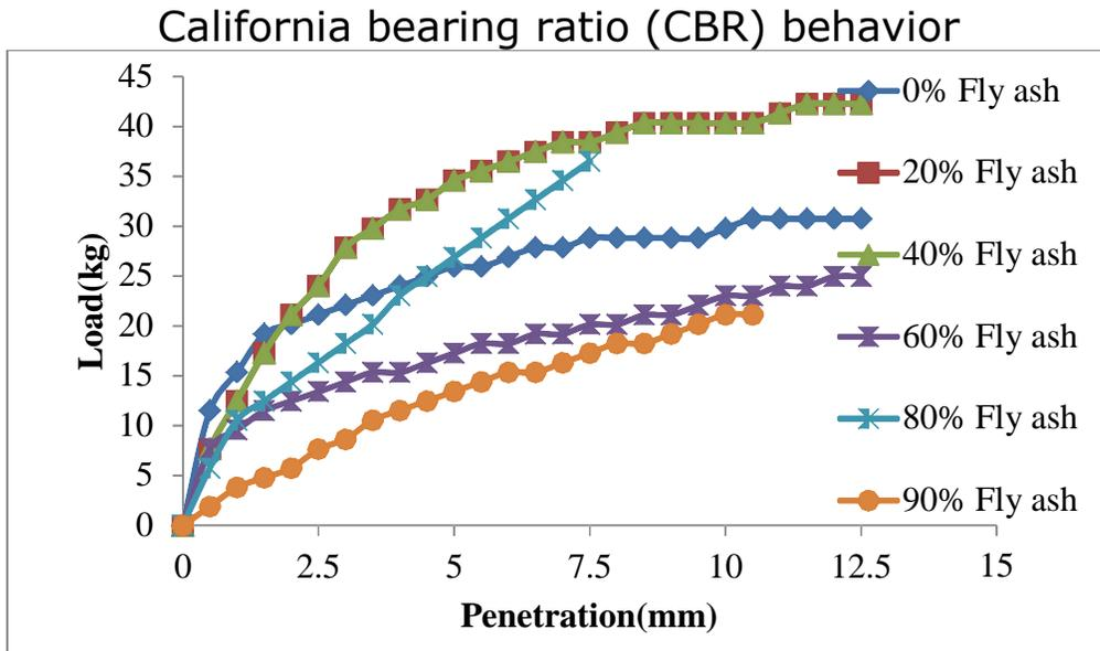
Figure 17: Soaked CBR test result expansive soil mixed with various proportion of fly ash
