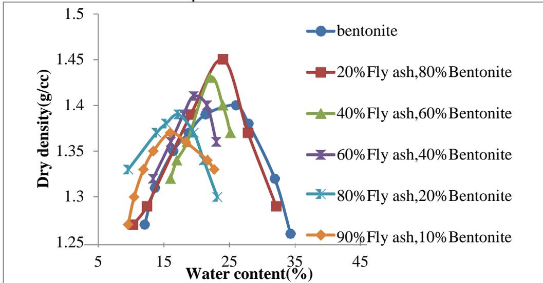
Figure 10: Standard Proctor Compaction test of expansive clay stabilized with fly ash
