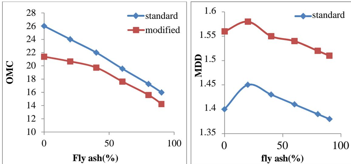
**Figure 12:** Variation of OMC with fly ash% **Figure 13:** Variation of MDD with Fly ash %
