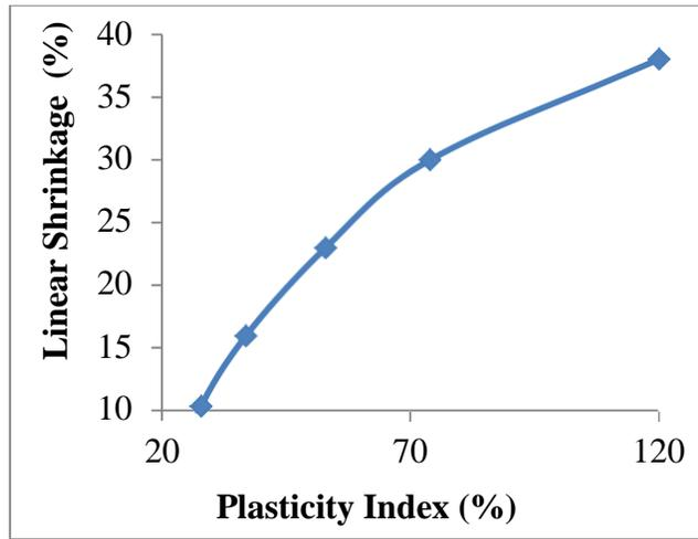
**Figure 7:** Variation of linear shrinkage with PI (%)
