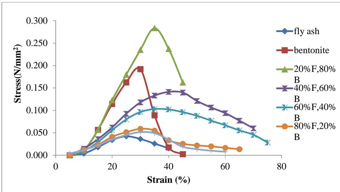
Figure 15: Unconfined compressive strength test result at modified proctor density
