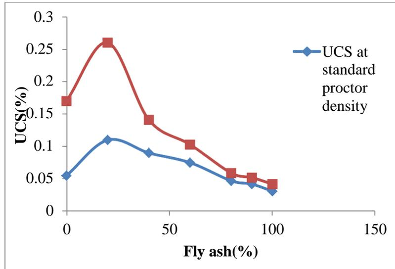
**Figure 16:** Variation of Unconfined compressive strength with fly ash content
