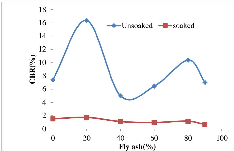
**Figure 19:** Variation of CBR (%) of expansive soil treated with fly ash
