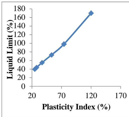
**Figure 4:** Variation of liquid limit with PI (%)
