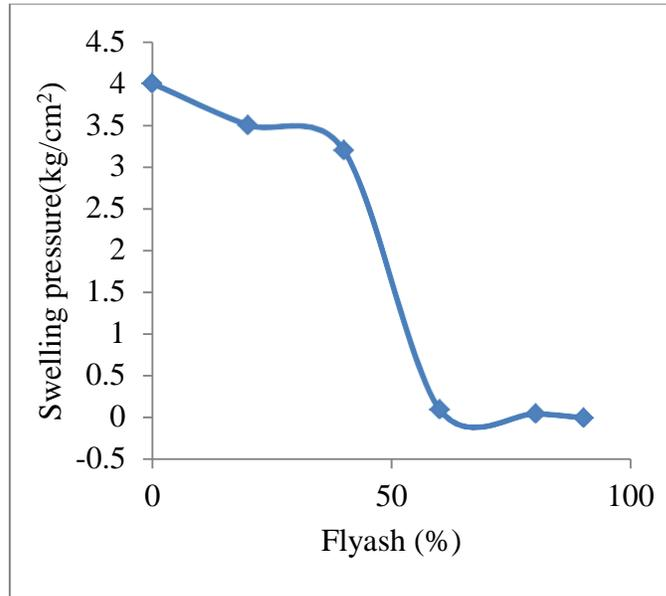
**Figure 8:** Effect of fly ash on swelling pressure of clay
