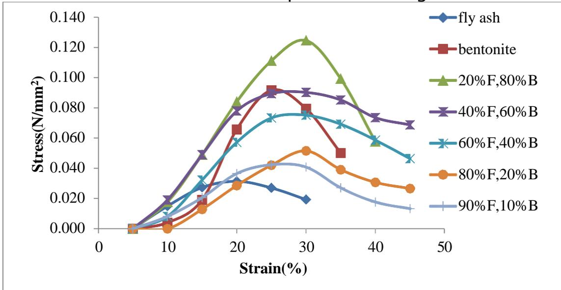
Figure 14: Unconfined compressive strength test result at standard proctor density
