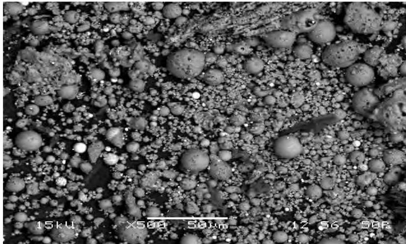
**Figure 2:** Particle arrangement (SEM) at 500M: Flyash
